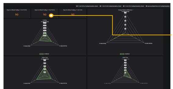
Data driven maintenance decision based on days to critical fouling. Here giving plenty of lead time to plan maintenance activity in advance
